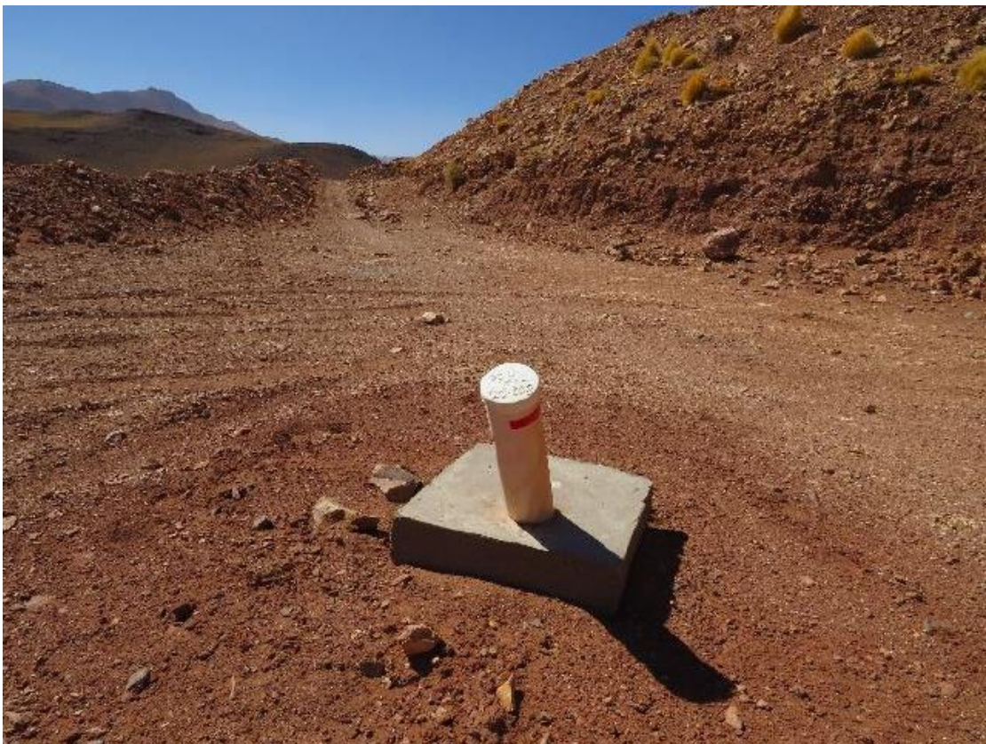
Figure 20-3: Platform DDH-20-008 cleaned and rehabilitated
