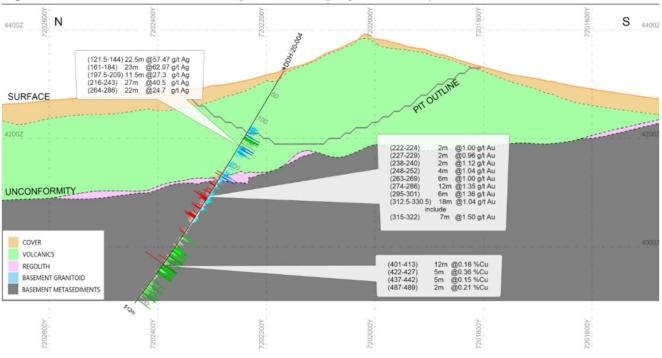
Figure 2 - Cross-Section 8525 (Looking East) with Highlighted Intercepts in Hole DDH 20-004
