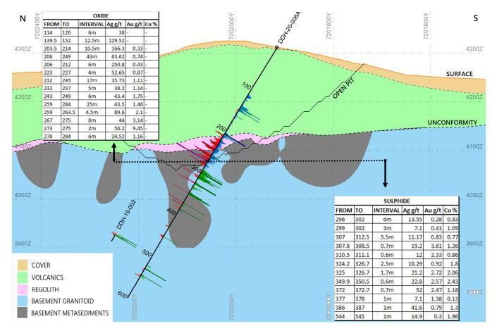
Figure 4 – Cross-Section 8350 (Looking East) with Highlighted Intercepts in Hole DDH 20-006
